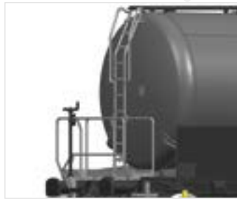
Delicate shunter's platform and ladder designs
