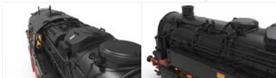
Separately applied tank lines, valves and grids over driver's cab
