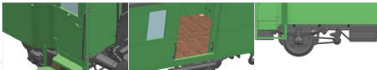
Delicate details such as separately-attached handrails, loading compartment floor with wooden structure
